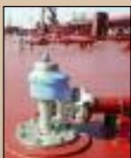
Fixed installed tank cleaning machines
